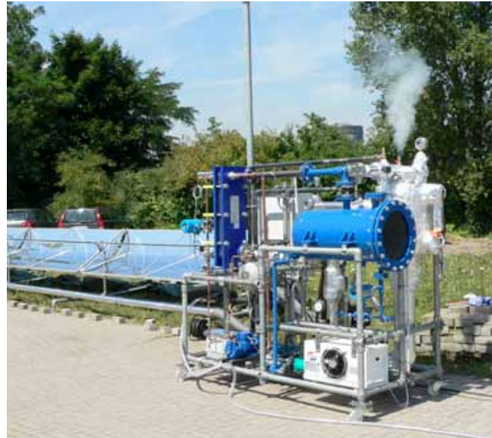
Solar thermic cold water generator with parabolic trough collector system and steam jet ejector chiller
