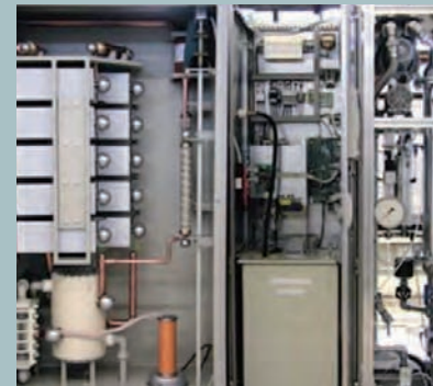
Opened pilot plant for the treatment of cloudy waste water using electronic impulses. On the left: lattice network high voltage pulse generator producing square wave pulses lasting 1 \mu s, with an amplitude of 60 kV and a repetition frequency of 10 Hz. In the middle: high voltage power supply for the impulse generator. On the right: generation of compressed air for the high voltage switching spark gaps.
