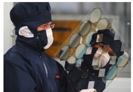
OLED panel light for general lighting.
